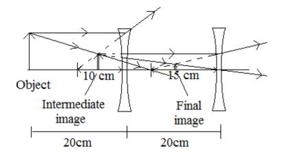
(b) First find the position and magnification of the intermediate image:
